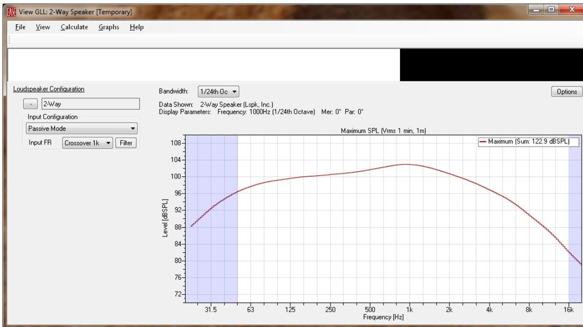
Figure 2-164 – Calculated maximum SPL with the 1 kHz crossover
