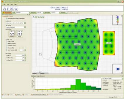
EASE Address v1.1 calculates 2D maps of both signal-to-noise and direct sound coverage.
